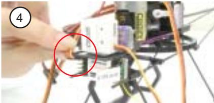
4. Plug in channel 1 for aileron servo.
